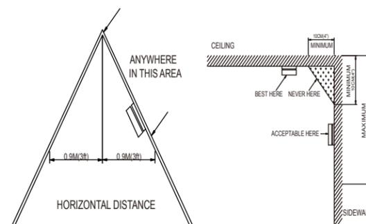
1. Near appliances or areas where normal combustion regularly occurs (kitchens, near furnaces, hot water heaters). Use specialized smoke alarm with unwanted alarm control for these areas.
