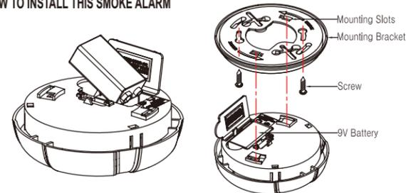
**WARNING:** Smoke alarm installation must be in accordance with the requirements of any national and local codes that may apply.
